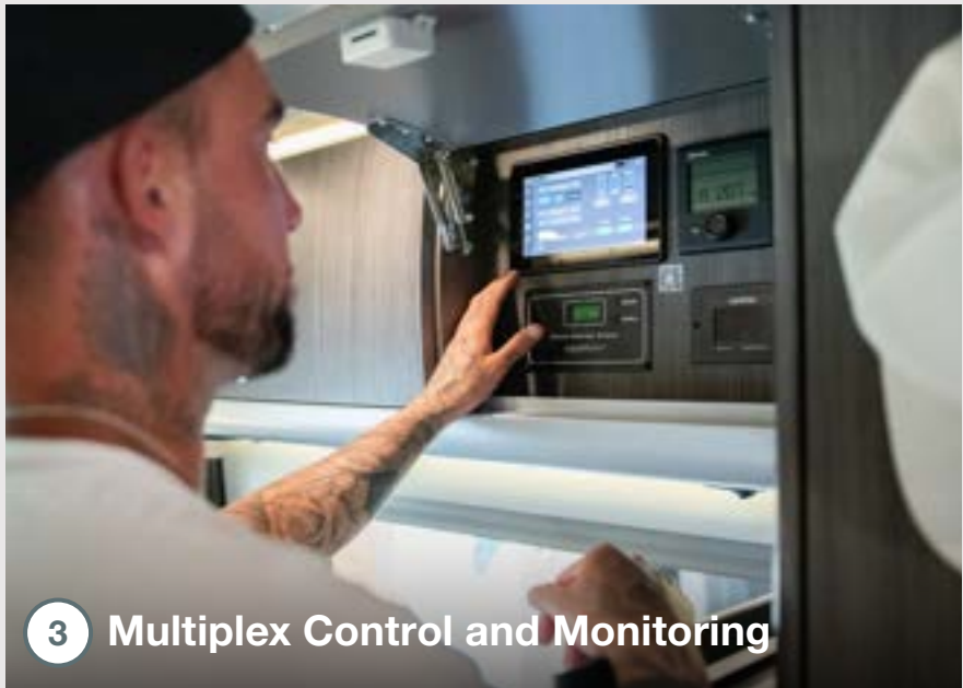
3 Multiplex Control and Monitoring Control shades, A/C, lighting and monitor tanks and power levels
